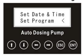
— On the main interface, Press "ENT" to enter setting menu. Press "↑" or "↓" button, select the "set program" when "<" point to "set program" press "ENT" to "Select Pump set".</p>
