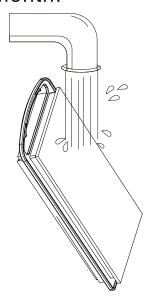
• Wash the entire motor monthly. Clean the inside of the motor with a pipe brush and place it back in the opposite direction.
