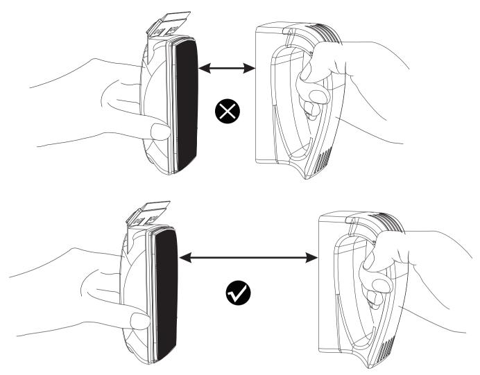
To attach the cleaner to the aquarium glass, first hold the part with the stiff cleaning bristles against the inside and the part with the soft surface against it, offset a little. Hold both parts firmly so that the glass is not accidentally damaged. Then, carefully push both parts together slowly until the magnet grips. Then you can start with the cleaning work.
